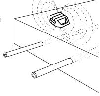
Estimating line depth using the C.A.T4+/eC.A.T4+/gC.A.T4+ and Genny4
