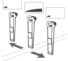
and forth across the maximum readout position, the cable or pipe's position can be pinpointed. The tidemark feature hold the maximum bargraph reading to ease identification of a peak readout.
