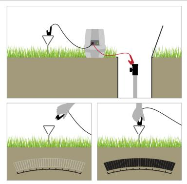
NOTE If it is not possible to use the Earth Stake use a nearby metal fence post, manhole cover or gully cover.
