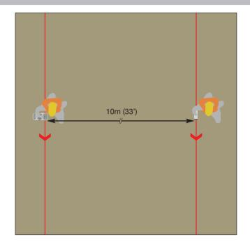
**NOTE** It is important to maintain the same distance and between the Locator and Signal Generator/Transmitter at all times. **NOTE** Only metallic services that are approximately in line with the Signal Generator/Transmitter orientation will be energised with a signal. Metallic services that are crossing the line of the Signal Generator/Transmitter will NOT be energised.
