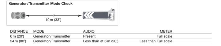
The SGV4 Signal Generator and MXT4 Transmitter have an in-built Self Test feature that automatically tests the Locator's circuits and transmitting aerials for correct performance each day (see pages 24-25). A Self Test can also be initiated manually by holding down the Pulse/Continuous button while the Signal Generator/Transmitter is switched on.
