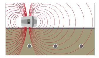
**NOTE** The signal will be radiated up to 3 m (9'9") either side of the Signal Generator/Transmitter but NOT directly below when the Signal Generator/Transmitter is on its side.
