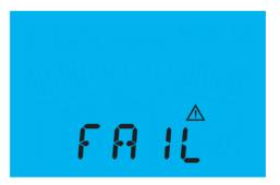
After any Self Test fail, the Signal Generator/Transmitter will automatically initiate a new Self Test when it is next switched on.
