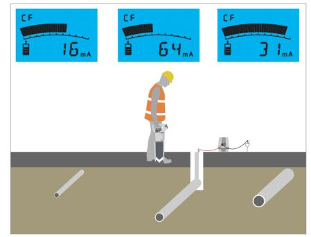
Signal Current Measurement can also help to identify the layout of pipe and cable networks as the main line after a 'T' will have most of the Signal Current remaining on it whereas the shorter connection will have correspondingly less.
